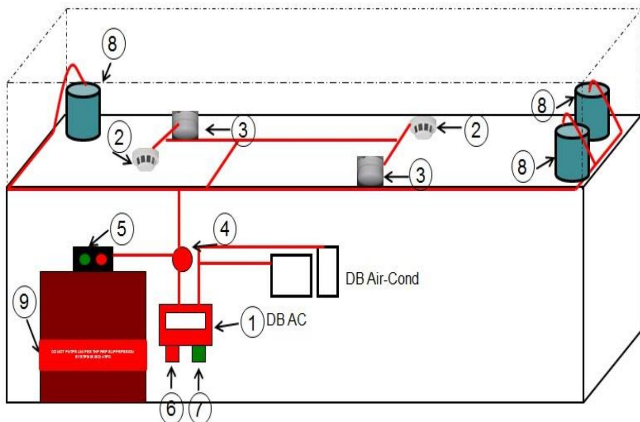
Note: This is base installation for cabin size 6m x 6m x 3m(H)
